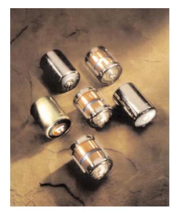
The SM-4 digital-grade geophone element is designed for low weight, long field life and ultra-reliable performance. Precision engineered components and computerized test equipment ensure consistency in manufacture and operation throughout and beyond the replacement guarantee period of 3 years.
