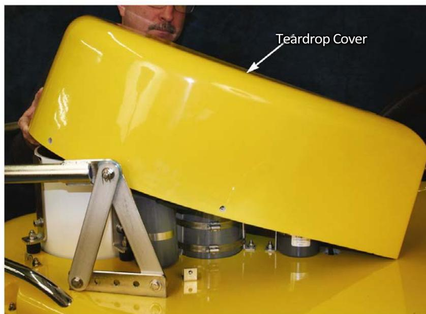
*Figure 4-5: Removing the Teardrop Cover*
