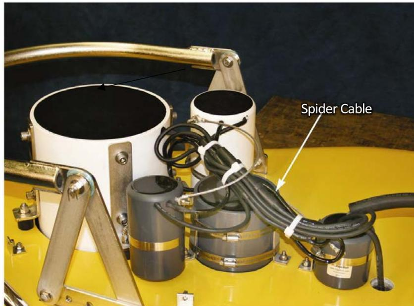
*Figure 4-6: Teardrop Cover Removed*
