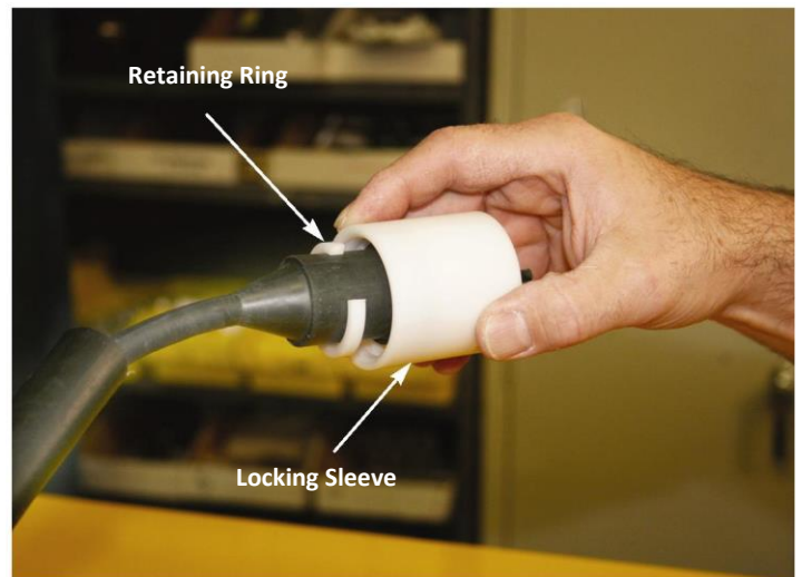
Figure 4-2: Retaining Ring and Locking Sleeve Removed
