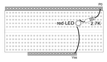
Figure 10 - Blinker circuit on breadboard
