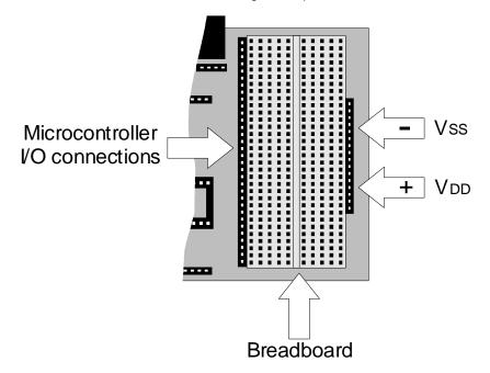
Figure 4 - Typical Prototyping Area
