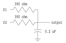
Figure 14 - Filter/combiner for DTMFOUT2
