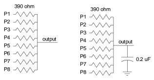
Figure 19 - Combining outputs for SOUND8
