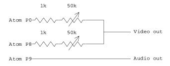
Figure 21 - Video output connections
