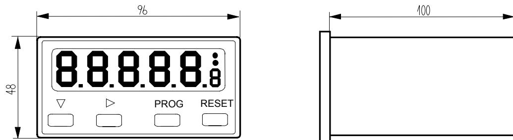
sectional view of switchboard: 45+0.3 mm x 92+0.3 mm, panel max. 12mm
