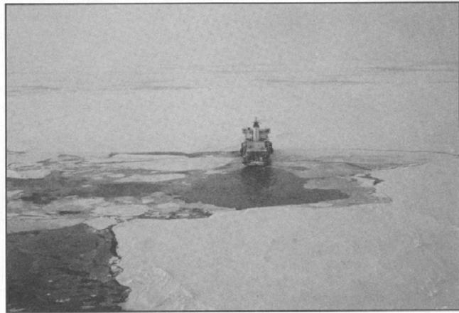
Oden during the 1991 station-keeping test.
