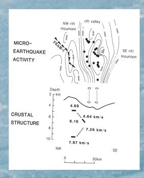
recording of microearthquake swarm occuring at the spreading center while the ice station drifted over the crestal mountain to the north
