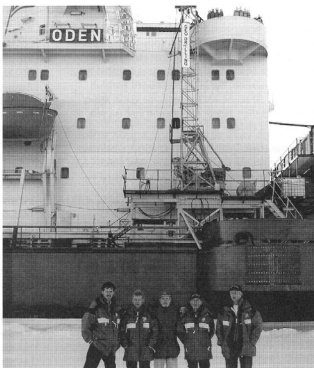
The drill rig mounted on Oden on the starboard side.
