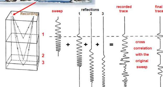
The vibrator generates a known signal which is cross correlated with the recorded trace to obtain a zero phase image of reflecting interfaces
