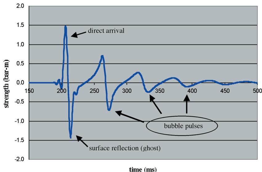
Figure 2. Signature of a single 40-in<sup>3</sup> air gun as recorded by a hydrophone 300 m below the gun.
