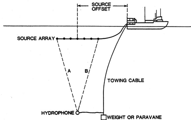
Figure 5. Equipment configuration for a far-field signature measurement. For a typical array, distance A = 300 m.
