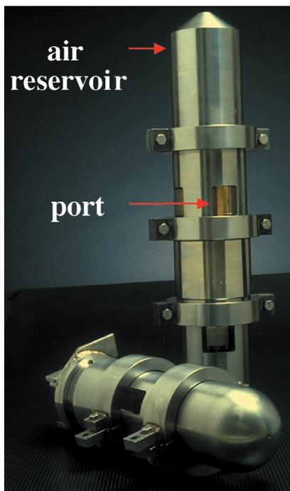
Figure 1. Two typical internal-shuttle air guns.
