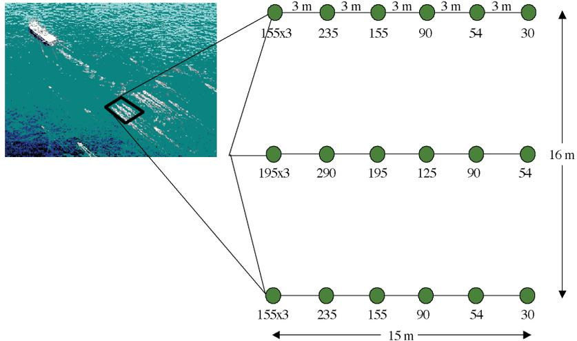
**Figure 4. Plan view of typical air-gun array. Numbers below the gun stations (green circles) are gun volumes (in<sup>3</sup>). The 155 × 3 notation indicates three guns, each with a volume of 155 in<sup>3</sup>, so close together that their air bubbles coalesce after the guns fire. Such so-called "cluster guns" produce sound more efficiently than a single large gun. (Figure courtesy of Schlumberger).**
