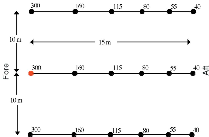
**Figure 7. Plan view of the air-gun array used for the modeling study. Numbers next to each gun site are gun volumes (in<sup>3</sup>). Red circle marks the origin of the coordinate frame.**
