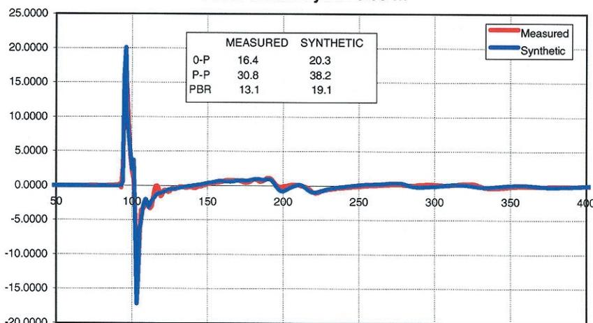
**Figure 6. Comparison of measured and modeled signatures for a small air-gun array.**
