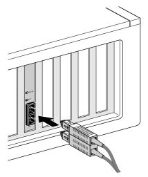
3 Connect the other end of the cable to an active 100BASE-FX Fast Ethernet network port.
