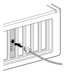
2 Connect the other end of the network cable to an active network port.
