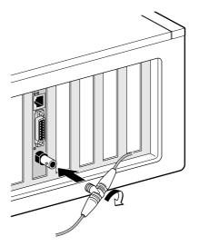
2 Connect the other end of the network cable to another PC or to a 50-ohm terminator.
