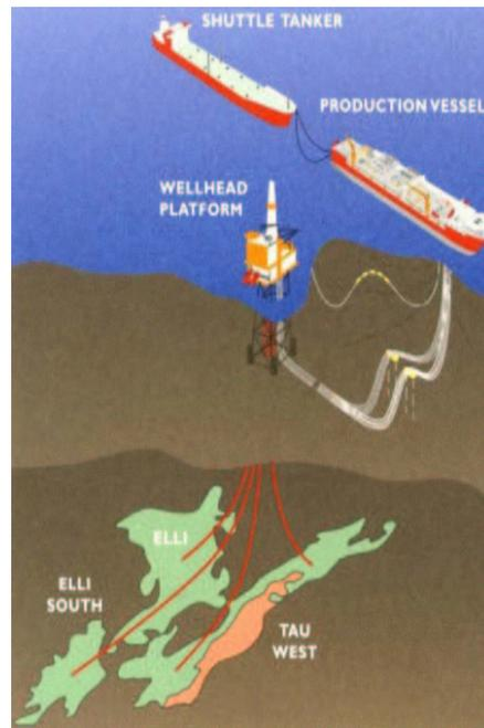
Figure 6.2: *Jotun is developed by a wellhead platform, tied back to a floating production vessel. Oil will be exported by shuttle tankers (Dick & Guargena, 2002).*
