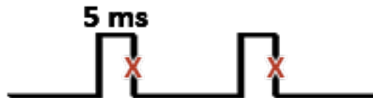
Figure 2-40: TTL - Negative Edge Trigger of 5ms (minimum)
