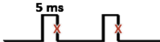
Figure 1-1: TTL - Negative Edge Trigger of 5ms (minimum)
