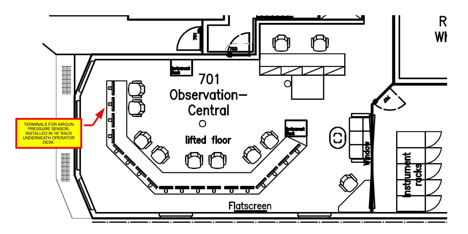
Location of terminals for pressure sensor display - monitoring of airgun pressure. GA drawing version: 08-6543-00-101-001-General\_Arrangement\_v7\_44.pdf
