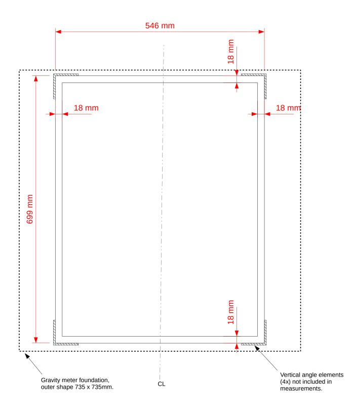
Gravity meter S/N: S-99 frame dimensions, for foundation. Department of Earth Science, University of Bergen, Norway 29 July 2016 (O.M.)
