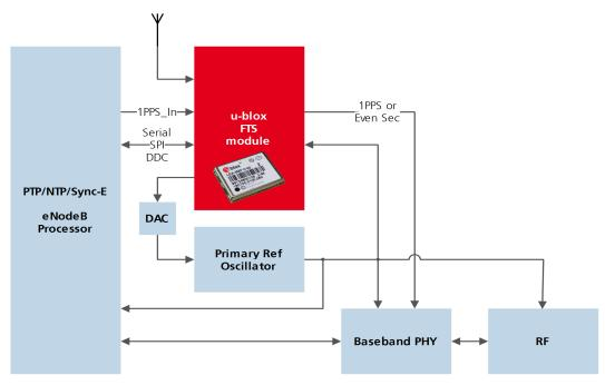
In this use case, the FTS device disciplines an external oscillator via an external DAC. During holdover the input to the external DAC is frozen and the phase of the time pulse output is maintained by the primary reference oscillator, but only guaranteed to be fully coherent with the internal oscillator. The FTS receiver can also be commanded to perform a one-off calibration of the tuning slope of external oscillator if necessary.
