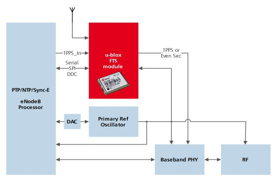
The frequency offset of the external oscillator is measured by the FTS device and communicated to the host which can then make any corrections necessary. The FTS device also generates a PPS phase reference internally (with no guarantee of coherence with the external oscillator). During holdover, the phase of 1PPS signal is maintained using either the primary reference oscillator or the 1PPS\_In signal, according to their respective uncertainty.
