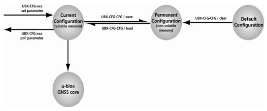
It is possible to change the current communications port settings using a UBX-CFG-CFG message. This could
