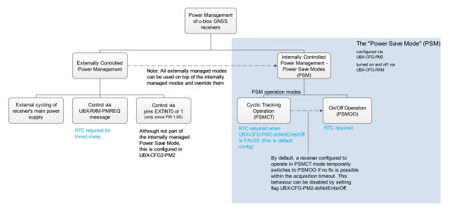
The majority of the Power Management section is detailing the Power Save Mode (Internally Controlled Power Management). However, some the concepts relevant to the Externally Controlled Power Management are detailed, such as the EXTINT Control, Wake up and Power On/Off Command.
