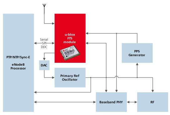
In this use case, the system PPS is generated by an external device from the output of the primary reference oscillator. The FTS receiver measures the phase of this PPS input against GNSS time or the best available source. Any small phase corrections necessary can be made by the receiver via adjustments to the oscillator frequency or directly by the host to the PPS generator (e.g. to accelerate removal of large phase errors). During holdover
