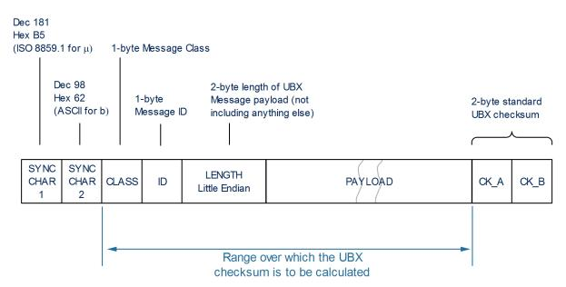
The checksum algorithm used is the 8-Bit Fletcher Algorithm, which is used in the TCP standard (RFC 1145). This algorithm works as follows:
