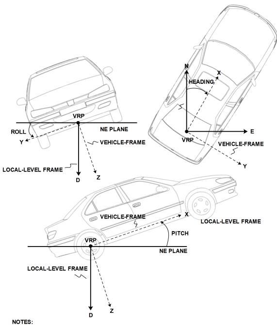
NOTES: N = NORTH, E = EAST, D = DOWN, IMU-FRAME ALIGNED WITH VEHICLE-FRAME
