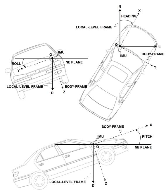
NOTES: N = NORTH, E = EAST, D = DOWN, IMU-FRAME ALIGNED WITH BODY-FRAME
