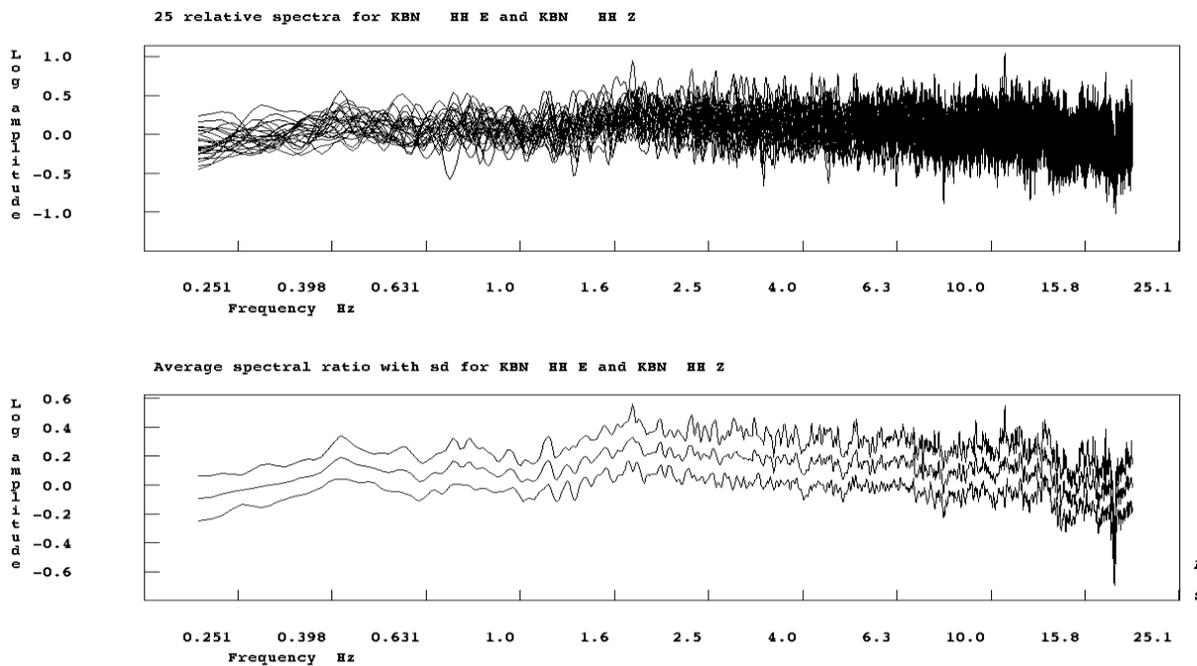
Figure 5 Example of a H/V ratio for station KBN. The top figure shows 25 relative spectra and the bottom figure is the average with standard deviation of the 25 spectra.
