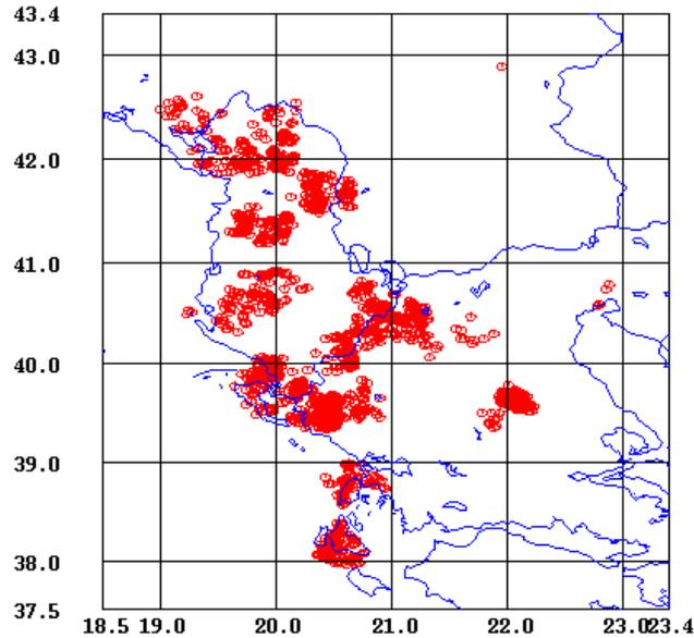
Figure 4 The midpoints between stations and events for calculated Q values.
