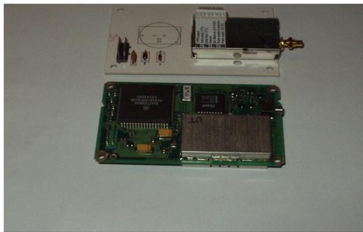
**This module it is a NMEA compatible 12 channel GPS receiver.**
