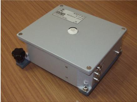
The SR97xx is a low cost compact and rugged 4.5Hz triaxial seismic sensor/digitizer. It allow to record seismic signal using low-cost geophones that can be embedded in the unit or placed at short distance.
