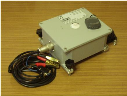
The SR04xx is a rugged and compact seismic system designed to recording signals produced by seismometers (geophones, velocity-meters, accelerometers, etc..). SR04 and its components make up a scientific instrument suitable for professional use and training purposes.
