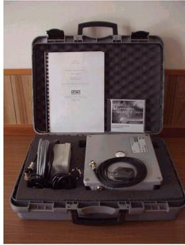
**This case is designed to allow an easy way to transport SL and SR 04 and 97 series of digitizers / dataloggers / sensors.**
