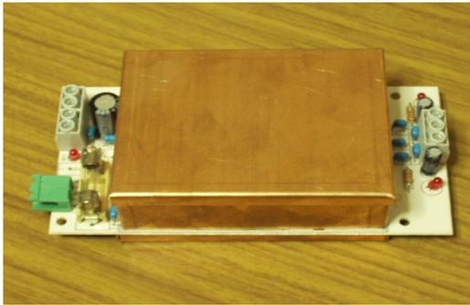
The SPOW10 is a power supply board designed to be used with the other seismic board of the SEISMOSTACK series. The unit is a switching power regulator.
