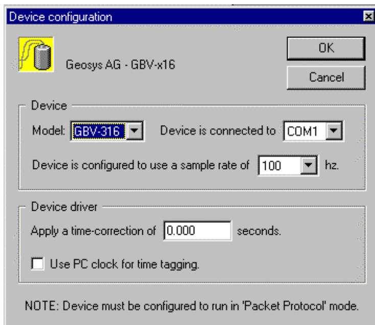
Figure 4 Example of digitizer setup
