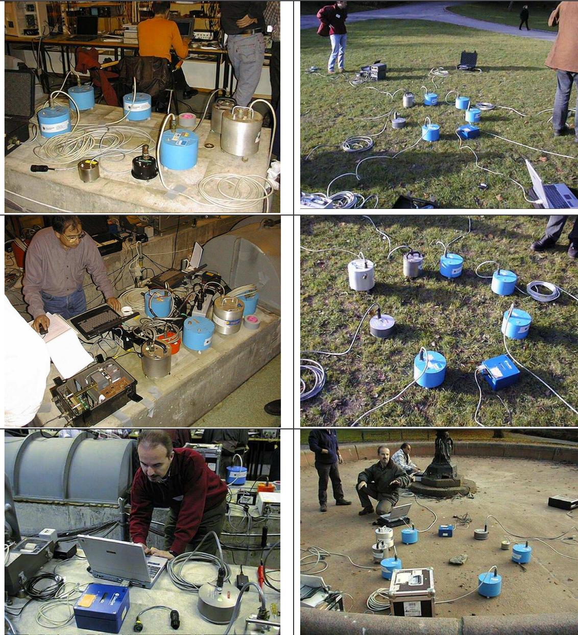
**Figure 1-1.** The different site locations used for the measurements. Figures on the left (top, middle and bottom) are from the laboratory. Figures on the right are from the free-field measurements (top and middle right: Site 1; bottom right: Site 2).
