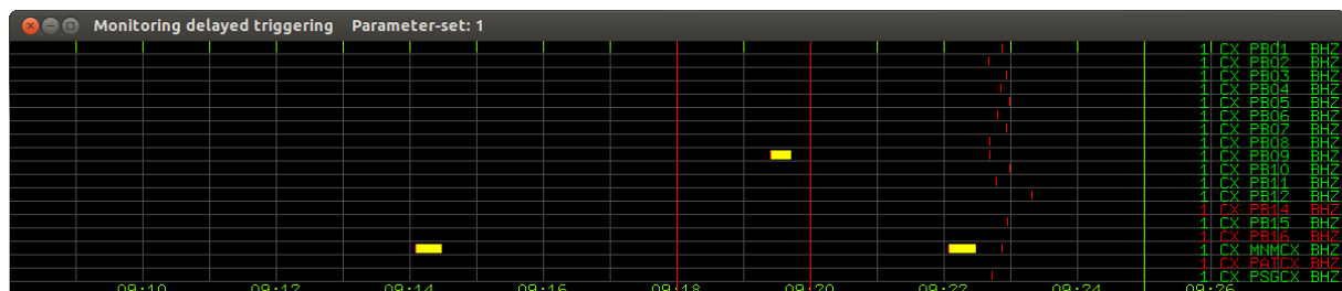
Figure 3.1 RTNET shows the signal from selected channels in “near-real-time”. It also indicates when channels are not transmitting data as for station PB14, PB16 and PATCX in this case. The red vertical lines indicate possible triggers, and are inserted when the traces are filtered. These triggers are not the RTQUAKE triggers computed by the RTDET module. Several instances of the program can be executed to show different stations, to apply different band pass filters, different color schemes, different window sizes and different positioning on the screen.
