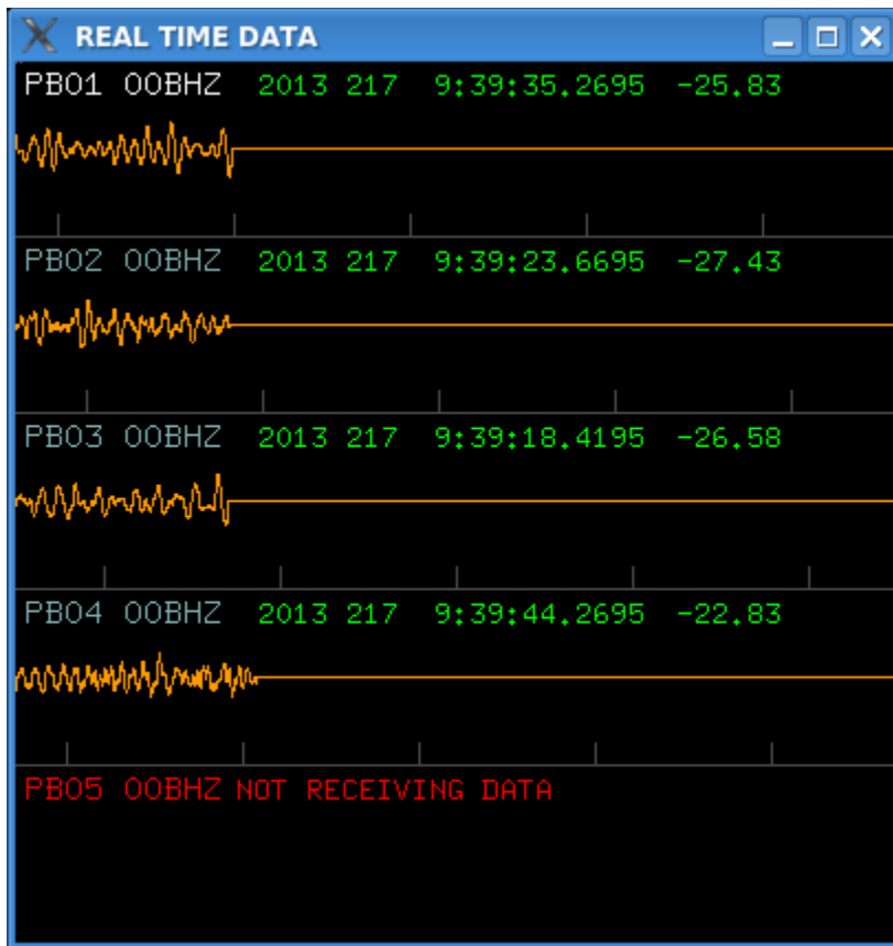
Figure 20 From command line: rtnet -n 5 -d -m 5 -x 400 -l DEMO1/streams_plot -f DEMO1/stations_plot 139.17.3.177:18000 Plot the first 5 channels in stations_plot file, textfield, 5 minutes x-axis and x-axis 400 pixels long.
