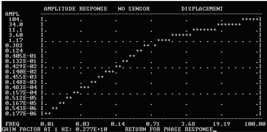
Figure 6.53: Making response file with poles and zeros.
