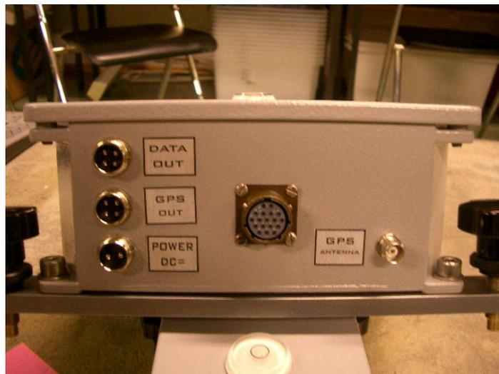
Figure 8. Digitizer connectors. Data out is RS232 to PocketPC, GPS out is not used and GPS is for the GPS antenna. The large connector is for connecting the sensors.
