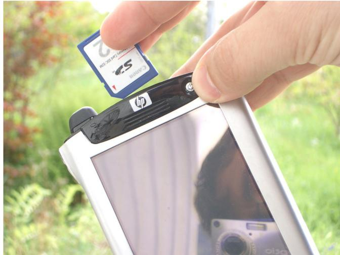
Figure 7. How to insert the SD card. Remember rounded corner lower left side.
