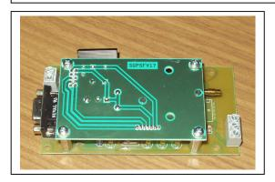
This module it is a NMEA compatible 12 channel GPS receiver and converter to the DCF77 pulsing code.
