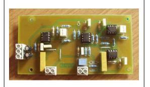
The SEQUA01.00 board is an electronic circuit that amplificates low frequency signals generated by a velocity sensor.
