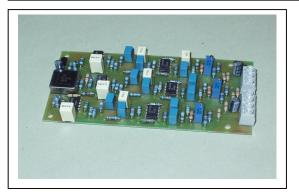
Strong motion sensor board with capacitive monolithic triaxial accelerometer.
