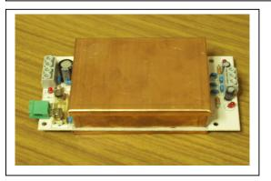
The SPOW10 is a power supply board designed to be used with the other seismic board of the SEISMOSTACK series. The unit is a switching power regulator.
