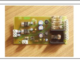
The SPOW10 is a classic linear power supply board designed to be used with the other seismic board of the SEISMOSTACK series. It is very simple and reliable even in operating and maintenance, if ever required. It is especially useful for training and evaluation purposes.
