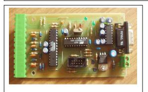
The SADC10 / 18 board series is a low-cost a/d converter for seismic measurements.
