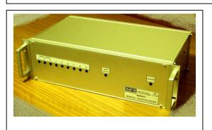
This rack is tipically used in building arrays where a number of digital sensors are to be connected to a single personal computer and/or datalogger.
