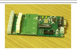
The SADC20 is a powerful, low cost and low noise a/d converter with 24 bit word resolution.
