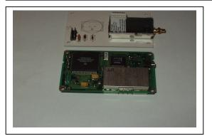
This module it is a NMEA compatible 12 channel GPS recevier.
