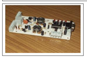
This transceiver device is a fully isolated RS232 – RS422 4 channel (2 channel full duplex) converter.
