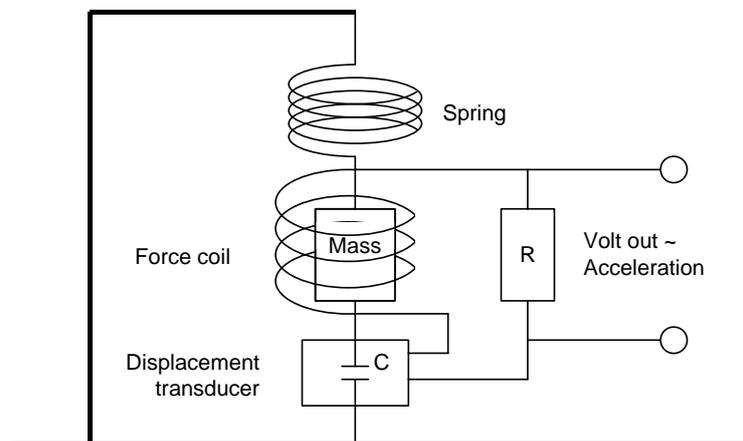
**Figure 1.4** Simplified principle behind Force Balanced Accelerometer. The displacement transducer normally uses a capacitor  $C$ , whose capacitance varies with the displacement of the mass. A current, proportional to the displacement transducer output, will force the mass to remain stationary relative to the frame.
