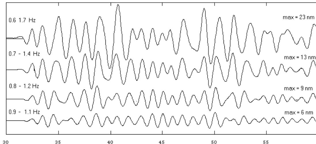
**Figure 3.2** The signal from Figure 3.1 band pass filtered with different filter widths. The signals have been corrected for instrument response to show displacement. The maximum amplitude in nm is shown to the right on top of the traces.
