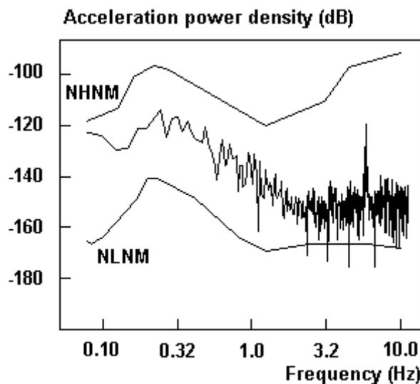
**Figure 3.5** Noise power density spectrum of the raw signal seen in Figure 3.1, top trace. The acceleration power is in dB relative to  $1 \text{ (m/s}^2\text{)}^2/\text{Hz}$ . The limits of the Peterson noise model is indicated (NHNM and NLNM). The spectrum has not been smoothed.
