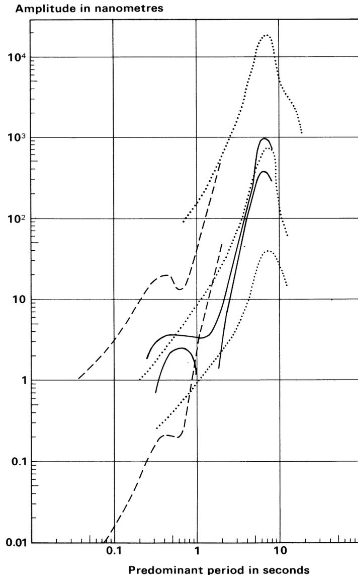
**Figure 3.3** Noise curves in rural environment. The 3 dotted lines correspond to the maximum, mean and minimum levels published by Brune and Oliver (1959), the dashed lines give two extreme examples observed in the US and the full line curves gives the limits of fluctuation of seismic noise at a European station on bedrock in a populated area 15 km away from heavy traffic (from Wilmore, 1979).
