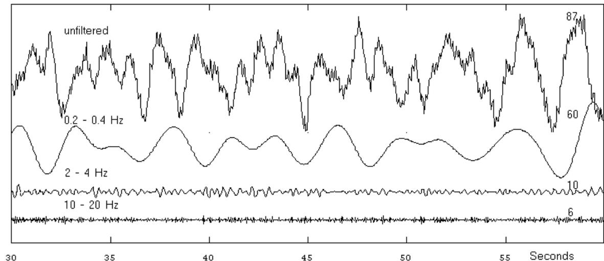
**Figure 3.1** Seismic noise in different filter bands at station MOL in the Norwegian national seismic network. The short period station (1 Hz) is situated about 40 km from the North Sea and the unfiltered trace clearly shows the high level of low frequency noise (0.3-0.5 Hz) generated by the sea. All traces are plotted with the same scale and the numbers to the right above the traces are the maximum amplitude in counts.
