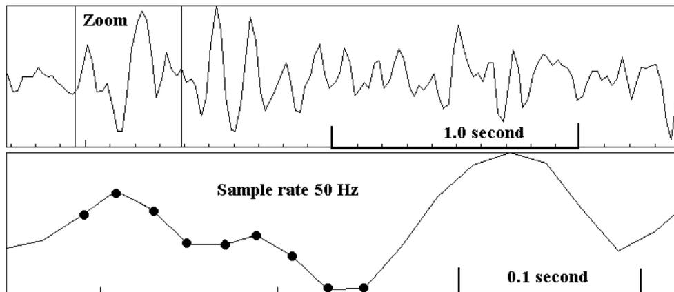
**Figure 1.5** Example of a digitized earthquake signal. The top trace shows the signal with a low time resolution and the bottom trace, the zoom window with a high resolution. In the zoom window, the discrete samples are clearly seen. The sampled points are indicated with black dots
