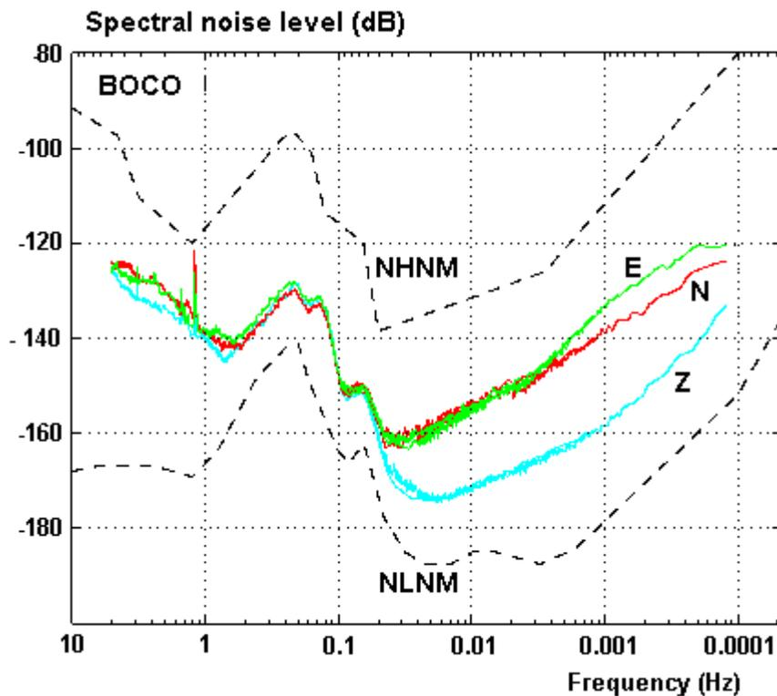
**Figure 3.4** The Peterson noise curves and noise spectral level for the IRIS station BOCO. The noise level is in dB relative to  $1 \text{ (ms}^{-2}\text{)}^2/\text{Hz}$ . The Peterson high and low noise models are shown with dashed lines. The noise spectra are shown for all 3 components. Note the lower noise level for the vertical (Z) component. Figure modified from IRIS station book (note that x - axis represents decreasing frequency).
