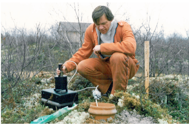
A short period sensor ready for installation
