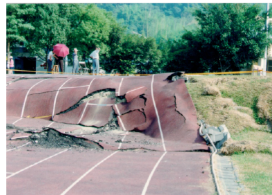
The picture shows a reverse fault rupture in connection with the destructive Chi Chi earthquake in Taiwan in 1999. The small picture shows close-up picture.
