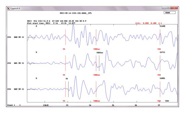
Three-component trace plot of station PFO at  $\Delta = 63.3^{\circ}$ , filtered 0.02-0.1 Hz: At this distance there is sufficient separation between S and SKSac to read both phases. The component codes of the horizontal components here are BH1 and BH2 to indicate that the instrument is not exactly aligned with the geographic directions. In this case, the direction of orientation is given with the component's metadata and can be used to rotate into a NS-EW system.
