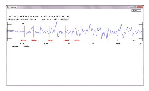
Vertical-component trace for station KMI at  $\Delta$ =154.0°, unfiltered: In this example we can see onsets that relate to the different travel-time branches of PKP. The corresponding depth phase times are also shown and phases are visible. Core phases are often most clear in the frequency band 1-5 Hz.
