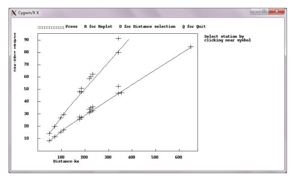
*Travel time plot*: We can also produce a simple travel-time plot that shows the observations (+) together with the calculated travel-time curves for P and S first arrivals according to the local velocity model implemented in the SEISAN location program (solid lines). For distances greater than about 150 km, our Pg (around the lower curve) and Sg arrivals (around the upper curve) come in mostly after the predicted first arrivals.
