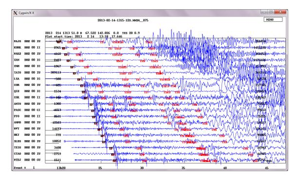
Multi-trace plot of vertical components, unfiltered: Plotted are the traces on which we have read the initial P. Based on the hypocenter obtained, we compute the synthetic arrival times of all phases. The traces are sorted by distance. The phases PP, S and SS are clear on all traces. We will now read the onset times of all these phases (plus P-wave first motion polarity), run the location program again with this additional information and see how the location changes.
