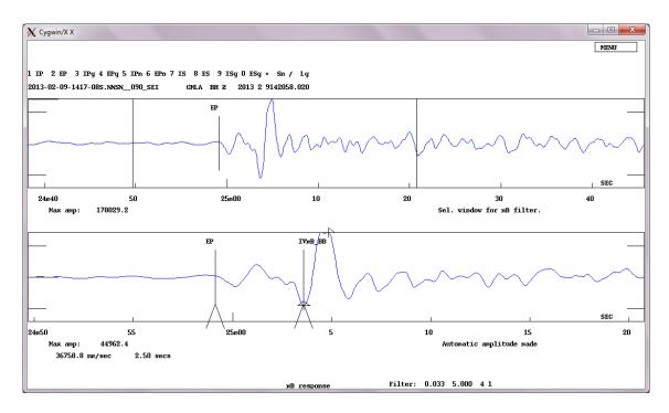
Amplitude reading for mB\_BB magnitude at station CMLA at  $\Delta$ =59.9°: As in the case of the regional event the amplitude IVmB\_BB is read on the bottom trace that has been deconvolved into a broadband velocity trace (top trace shows uncorrected data, which are in the case of a broadband seismometer also proportional to velocity): here 36758 nm/s with a period of 2.5 s.
