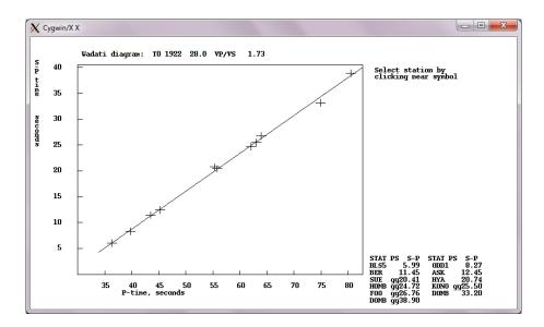
Wadati diagram: To check our readings we can plot the Wadati diagram (plotting S-P times against absolute P arrival times (labels on x-axis given to show scaling), and the data points should fall onto a line like in this example. Data points (+) that are significantly off the line should be checked and re-read.
