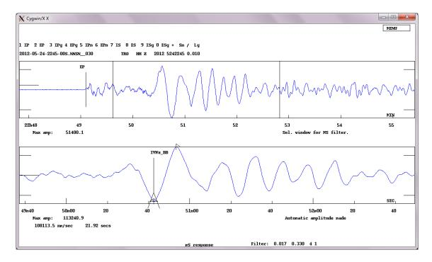
Vertical-component trace of station TRO at  $\Delta$ =5.3°, Ms\_BB filter: Ms\_BB can be used down to distances of 2°. This plot shows the Ms\_BB amplitude reading made for station TRO. The amplitude is automatically read between peak and trough, and stored as half of this measurement, which is 108113.5 nm/s with a period of 21.92 s. The computed magnitude is Ms\_BB = 5.7, compared to Ms\_BB = 6.1 for station ARU.
