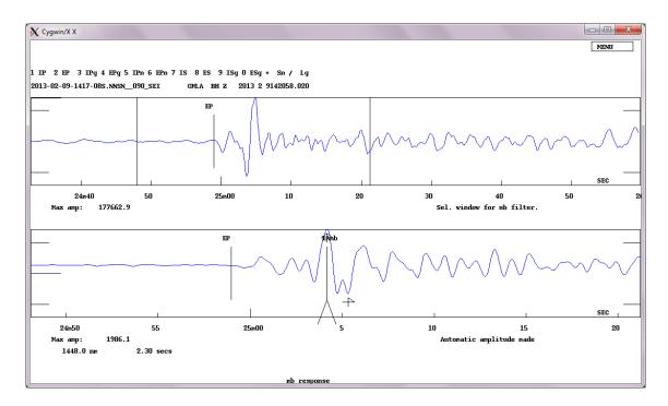
Amplitude reading for mb magnitude at station CMLA at  $\Delta = 59.9^{\circ}$ : As in the case of the regional event, the upper broadband trace is converted into a WWSSN short period trace (lower trace) on which the amplitude IAmb is read, here as 1148 nm with a period of 2.3 s.
