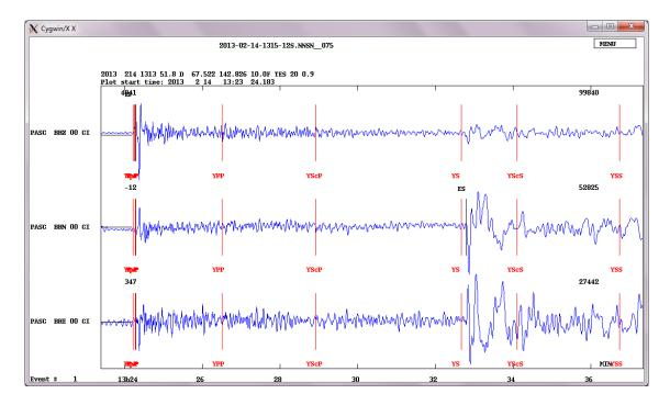
Three-component trace plot of station PASC at  $\Delta$ =62.2°, unfiltered: For this station P on the vertical component and S on the N component are very clear. Other phases are not very clear. Note that we do not pick the onsets at the calculated arrival times (red bars) but only at the distinct onset of the real phases with large SNR (black bars).
