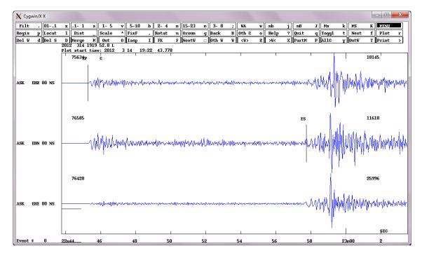
Three-component trace plot of station ASK at epicentral distance of 109 km, unfiltered: We normally read the S arrival on one of the two horizontal channels and not on the vertical as SP conversions may arrive prior to S and result in an incorrect reading of the onset time.
