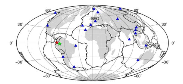
Map showing the epicenter of the Colombia earthquake (red star) determined by using a network of globally distributed stations (blue triangles). For comparison we plotted the epicenter from the single station (BFO, see label) 3-component location as a green star. For details of the BFO location see the next section.
