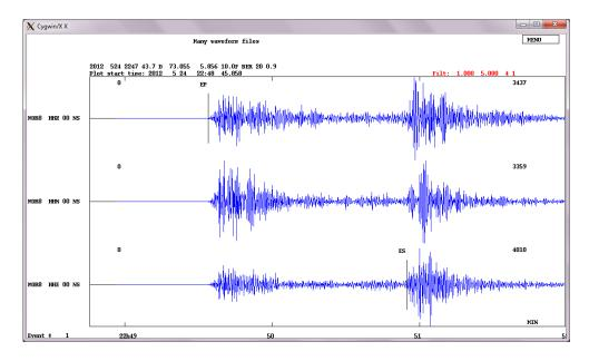
Three-component trace plot of station MOR8 at epicentral distance of 813 km, filtered 1-5 Hz: This is an example where the S arrival can be read quite well on one of the horizontal channels.
