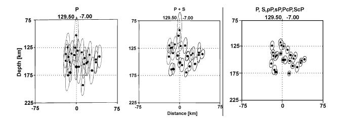
**Left:** hypocenter locations using only P phases; **middle:** by adding S phases; **right:** by adding also depth phases and core reflections. (Copy of Figure 7 from IS 11.1, modified from Schöffel and Das, J. Geophys. Res., Vol. 104, No. B6, page 13, Figure 2; © 1999, by permission of American Geophysical Union).
