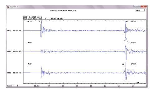
Three-component traces of station BLS5 at epicentral distance of 49 km, unfiltered: Plotted are the three-component broadband traces from the nearest station. P and S arrivals, and the ML amplitude were read. In this case the SNR was high enough so that it was not necessary to filter the broadband recordings to identify the phase arrivals.
