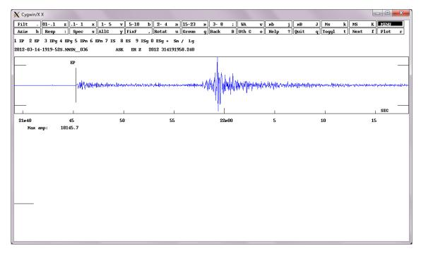
Single trace plot of station ASK at epicentral distance of 109 km, unfiltered: In SEISAN, we mostly do the phase picks on single trace plots, like shown here, or on three-component trace plots. For this recording on a short-period seismometer it is not necessary to filter the data in order to pick phase arrivals. The P arrival is marked.
