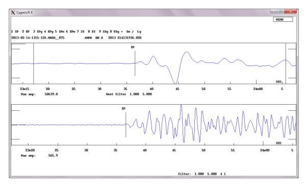
Vertical-component trace of station ANMO at  $\Delta = 65.4^{\circ}$ , unfiltered (top) and filtered 1-5 Hz (bottom): We start by reading the P arrivals that are very clear for this event. They can be read both on unfiltered (top) and high-pass filtered seismograms (bottom).
