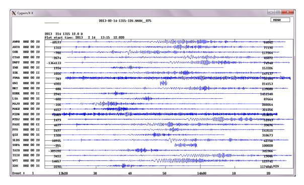
Multi-trace plot of vertical components, unfiltered: Record durations up to about 60 minutes at some stations and the observation of much larger surface-wave than body wave amplitudes hints to a large shallow earthquake at teleseismic distances.
