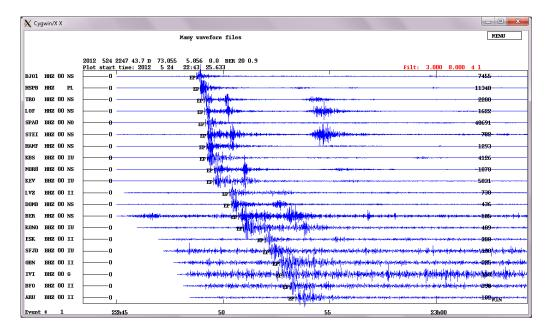
All vertical traces, filtered 3-8 Hz: We can see that the signal amplitude of the higher frequencies decreases as we go to larger distances due to attenuation. The distance range here is approximately 440 km (station BJO1) to 2960 km (station ARU).
