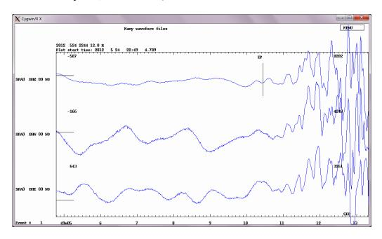
Three-component traces of station SPA0 at epicentral distance of 648 km, unfiltered: Zooming around the P arrival the phase can be picked with or without filter. The error on the phase reading here may be as large as 0.5 sec.
