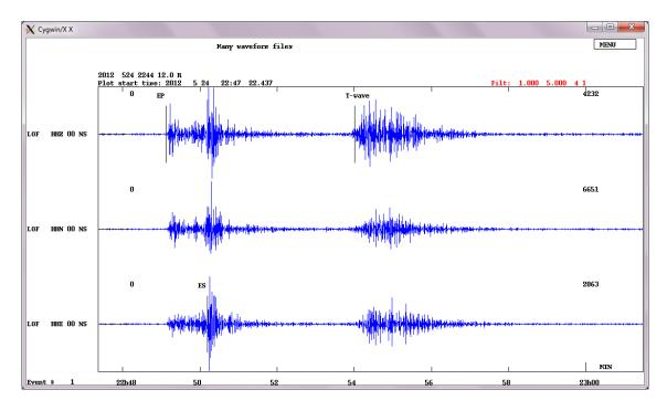
Three-component traces of station LOF at epicentral distance of 603 km, filtered 1-5 Hz: Looking at this coastal station, we clearly see the arrival of the T wave. The amplitude of the T wave is in this case comparable to the S-wave amplitude. According to the time difference (S-P)[in s]×10 the station is about 600 km away from the source.
