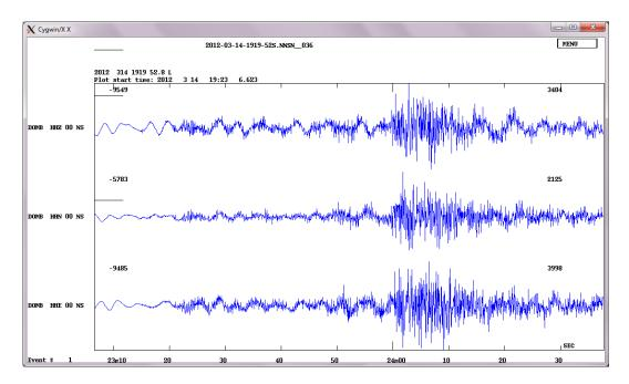
Three-component traces of station DOMB at epicentral distance of 342 km, unfiltered: Going to larger distances, the signal amplitudes at higher frequencies decrease relative to the more low-frequency microseismic noise, which peaks around 5 seconds. Here, we would normally filter the traces to read the phase arrivals.
