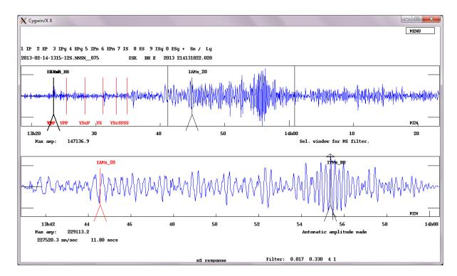
Traces of station ESK at  $\Delta = 54.4^{\circ}$ , Ms\_BB filter: Next we determine the two IASPEI standard surface-wave magnitudes. The bottom trace shows the reading position of the Ms\_BB amplitude IVMs BB (black arrow-bar) on an instrument corrected broadband velocity trace.
