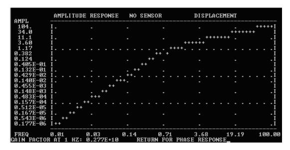
Figure 6.53: Making response file with poles and zeros.
