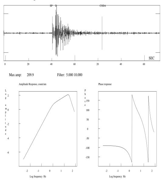
Figure 6.11: Plotting response curves
