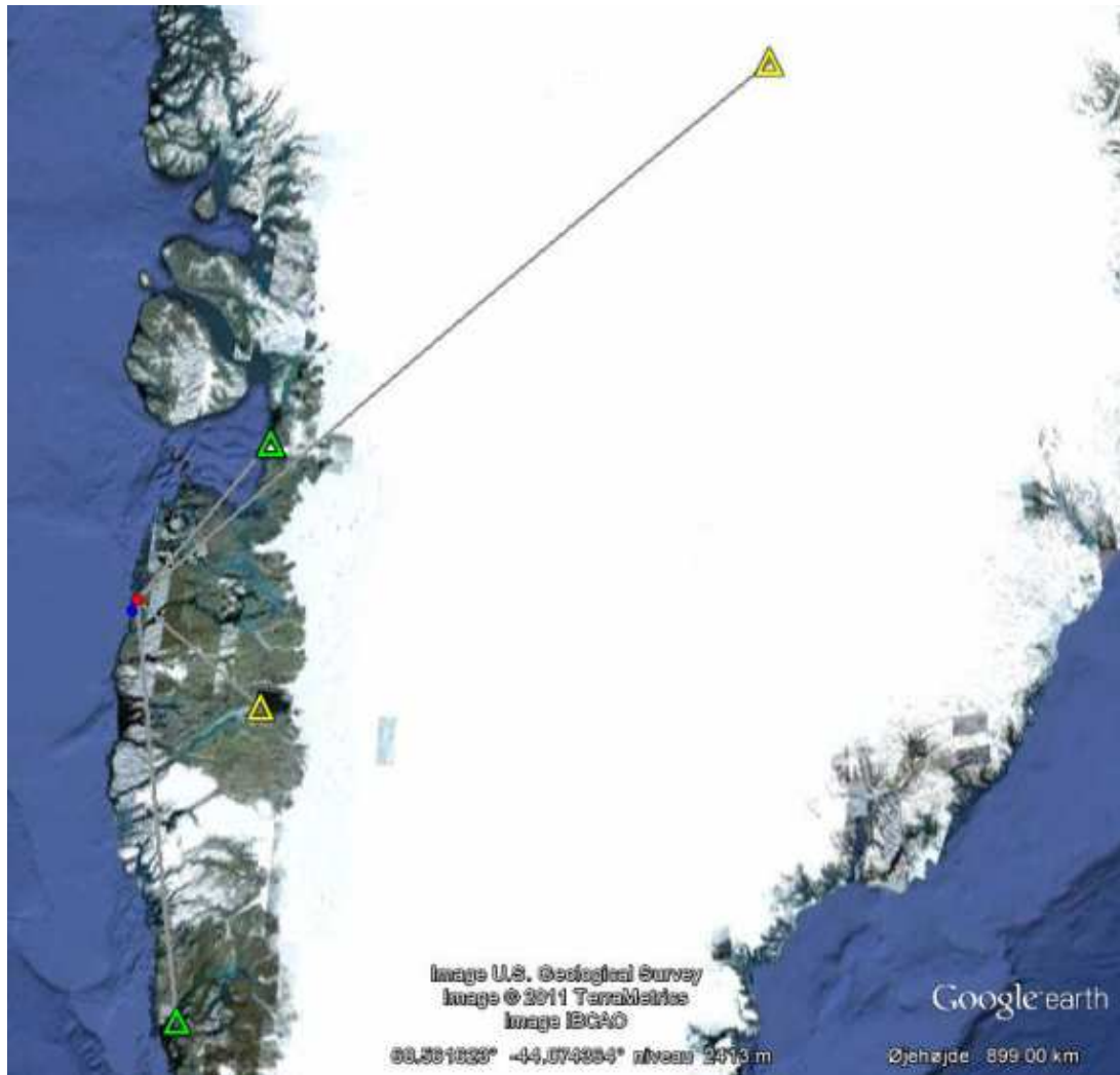
Figure 6.19: Example of automatic mapping with gmap. Earthquake in West Greenland. Blue dot is the old location and the red dot is the current location. Green and yellow stations are stations with good and ok residuals, respectively.
