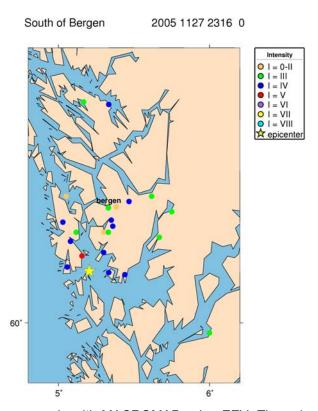
**Figure 52** Macroseismic map made with MACROMAP using EEV. The epicenter, taken form the S-file, is shown with the star.
