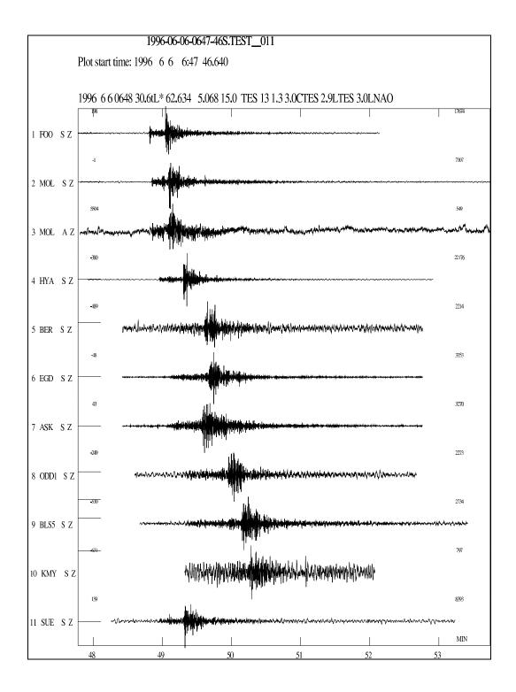
Figure 18. Examples of MULPLT with theoretical arrival times of some global phases. Short period seismograms are shown. The theoretical phases are marked with onset y below the trace and the read phases are marked normally above the trace.
