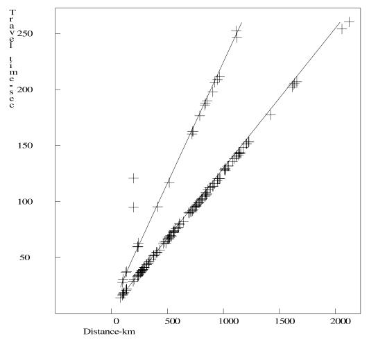
Figure 41. Example of travel time plot. Both P and S observed travel times are plotted with '+' symbol. Calculated times are shown by the solid lines, the lower one gives the first P arrivals, the upper line gives first S arrivals. The two outliers are observations from a station with incorrect timing.
