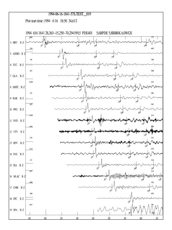
Figure 19. Example of MULPLT with theoretical arrival times showing global phases on a long period seismogram. The filter used from 0.01 to 0.1 Hz. Without filtering, almost nothing would have been seen on this broadband station.
