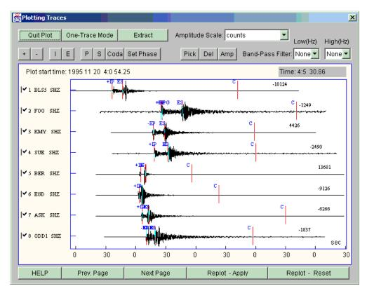
Figure 9. Plotting window. Multi-Trace mode
