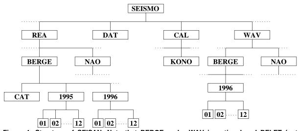
Figure 1. Structure of SEISAN. Note that BERGE under WAV is optional and DELET (not shown) under REA has a similar directory structure as e.g. NAO.
