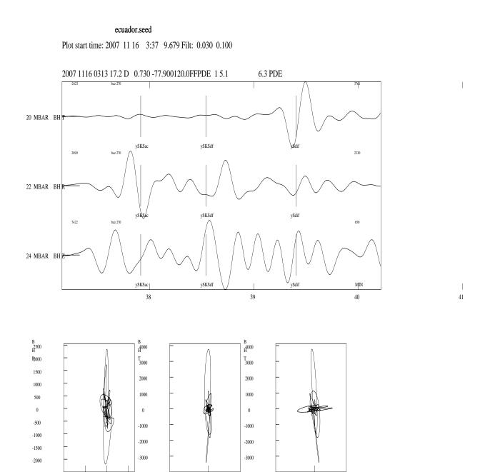
Figure 27 Example of particle motion plot.
