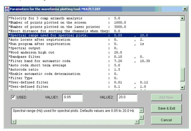
Figure 3. Edit Window of the configuration file: MULPLT.DEF
