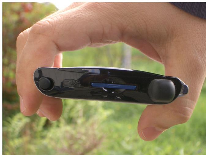
Figure 6. SD memory card inserted in the PocketPC.
