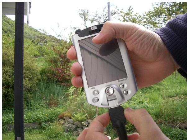
Figure 4. Release the USB/serial cable. Press the two buttons on the side of the connector.
