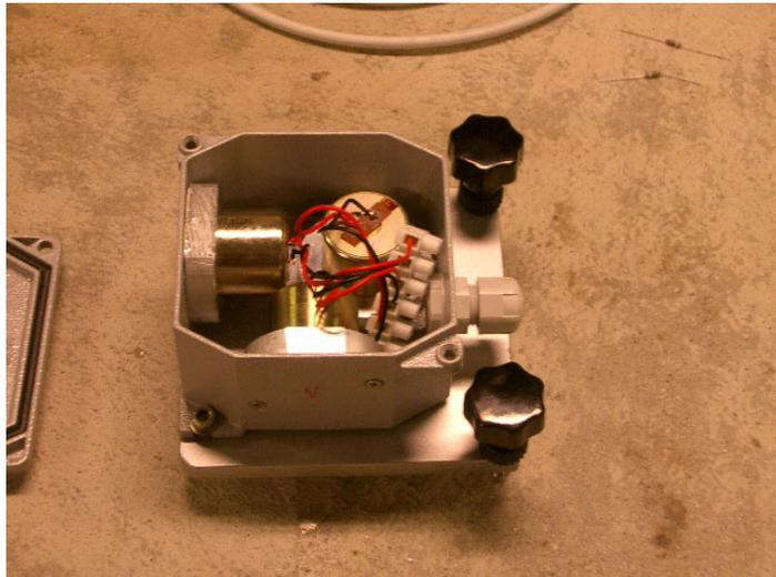
Figure 10. Sensor Housing. The housing is waterproof provided that the cable connection is tight.
