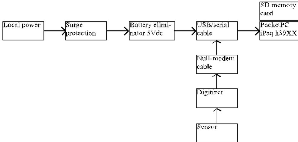
Figure 1. The different components of the seismological station.
