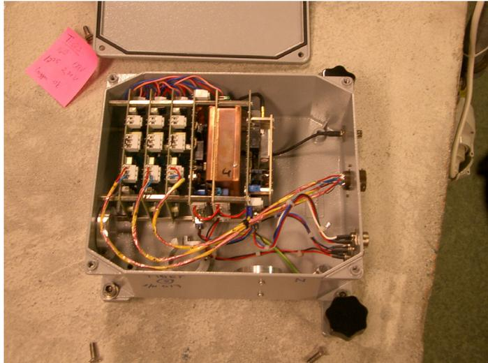
Figure 9. Inside Digitizer. The three cards to the left are amplifier and filter cards, then follows digitizer, power supply and GPS.
