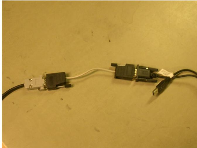
Figure 5. Null-modem cable connected between digitizer and PocketPC serial cables.
