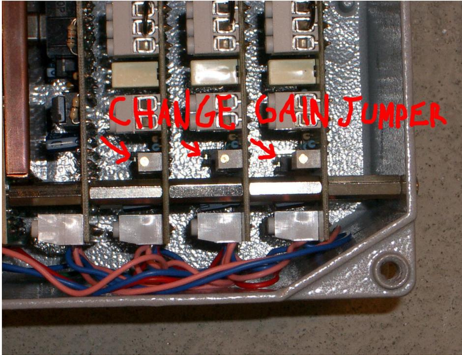
Figure 11. SADC10. Gain adjustment by changing jumper.
