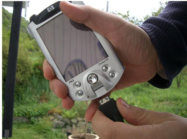
Figure 3. Insert USB/serial cable on PocketPC.
